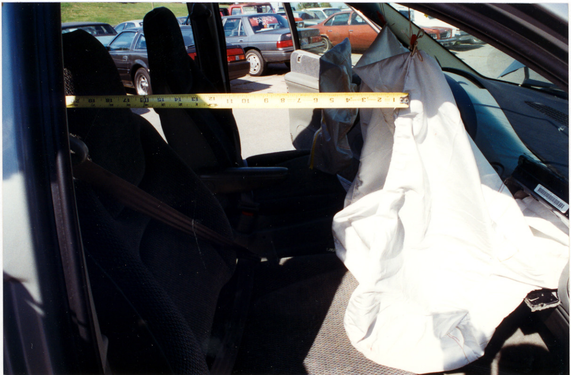
84. Longitudinal measurement of the seat relative to the deployed passenger side air bag.
